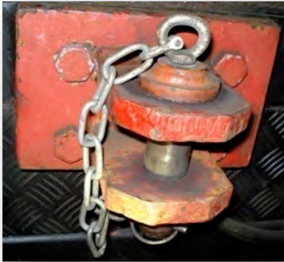
Figs. 5 & 6 Intact and damaged coupling points on the RGU
