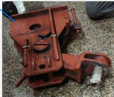
Fig 8 & 9 Damaged and intact coupler used to connect tow-bar to LU passenger train (note point of failure in image on the left)
