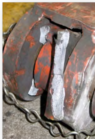
Fig. 4: Fracture face of the emergency coupler
