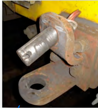
Figs. 5 & 6 Intact and damaged coupling points on the RGU
