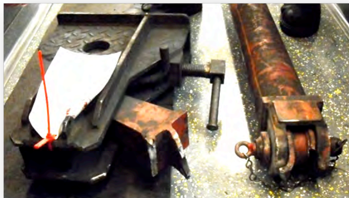
Fig 8 & 9 Damaged and intact coupler used to connect tow-bar to LU passenger train (note point of failure in image on the left)
