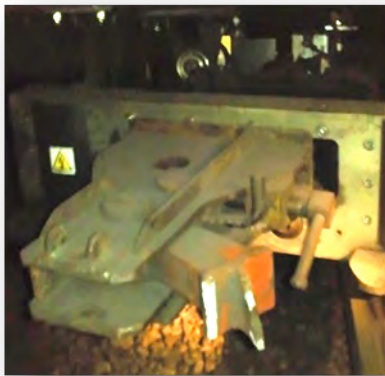
Fig 8 & 9 Damaged and intact coupler used to connect tow-bar to LU passenger train (note point of failure in image on the left)
