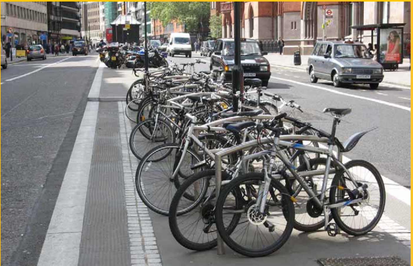
Along High Holborn, a widened central median has been used to provide additional cycle parking, as well as support pedestrian crossing movements.
